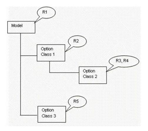
The callouts (i.e. "R1", "R2", "R3, R4" and "R5") denote the rules assigned at the different levels. For the rules assigned to the same node, assume that the rules are listed in the increasing order of priority value.
