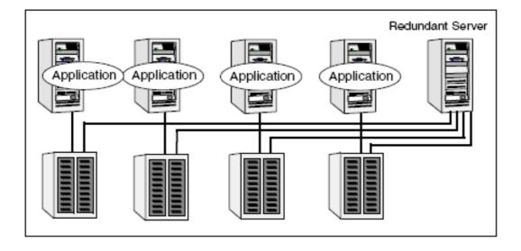
The exhibit shows an N-to-1 cluster configuration, in which nodes are connected to storage devices via dual-hosted SCSI cables.
