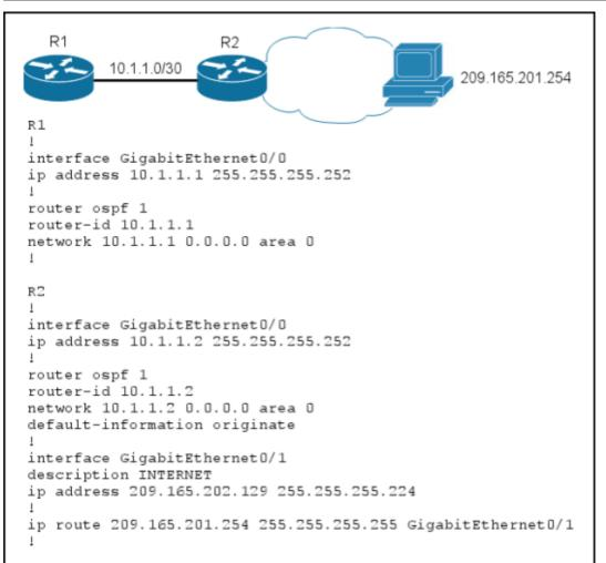
Routers R1 and R2 are configured as shown, and traffic from R1 fails to reach host 209.165.201.254.
