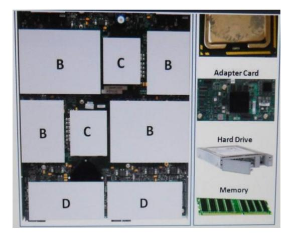
Refer to the exhibit The pictures on the right are the internal components of the Cisco UCS 6250 Blade Server Which component image should be applied to which empty component block?
