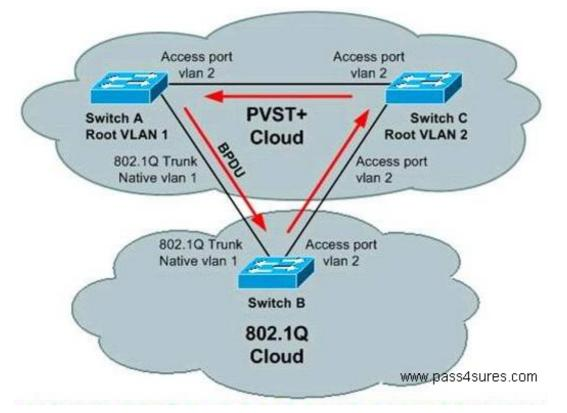
A. Switch A sends PVST+ BPDUs of VLAN 2 (to the SSTP address that is flooded by Switch B) towards Switch C. Switch C will put port C.B into a typE.inconsistent state, which prevents the loop.
