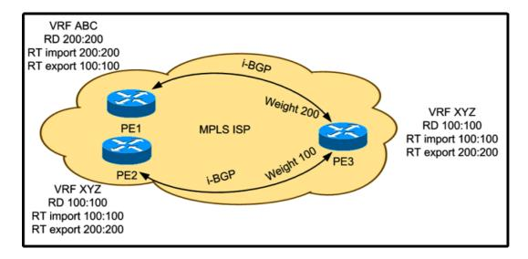
PE1 and PE2 are advertising the same subnet 196.168.10.0/24 to PE3. Which PE advertised subnet is installed at PE3 BGP table?
