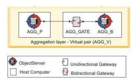
Anadministrator at Widgetcom intends to use the standard multitier architecture configuration that ships with IBM Tivoli Netcool/OMNIbus V7.4 (Netcool/OMNIbus) to deploy an aggregation pair of ObjectServers AGG\_P (primary) and AGG\_B (backup) with a failoverbidirectional gateway connecting them: AGG\_GATE.
