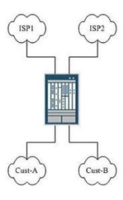
In the exhibit, Customer A and Customer B connect to the same SRX Series device. ISP1 and ISP2 are also directly connected to the SRX device. Customer A's traffic must use ISP1, and Customer B's traffic must use ISP2.
