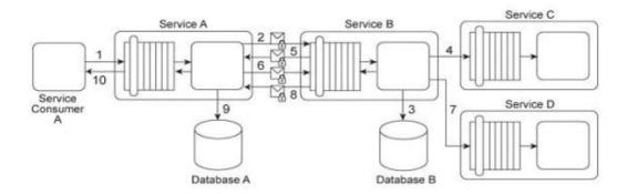
Services A and B use digital certificates to support message integrity and authentication. With every message exchange between the two services (2, 5, 6, 8), the digital certificates are used. It has been determined that both Databases A and B are vulnerable to malicious attackers that may
